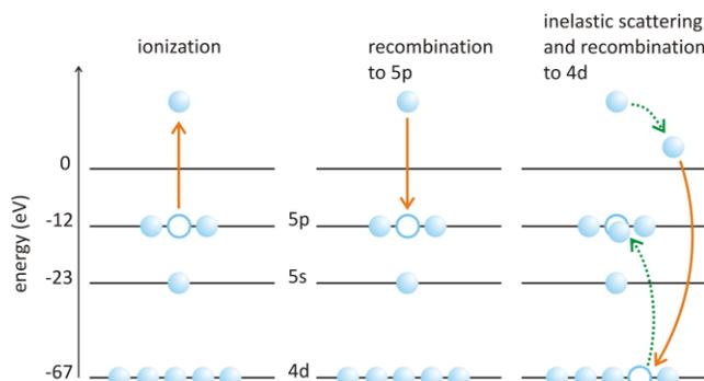
**Figure 2** sketch of the ionization and recombination steps of HHG (spin states are not considered).
