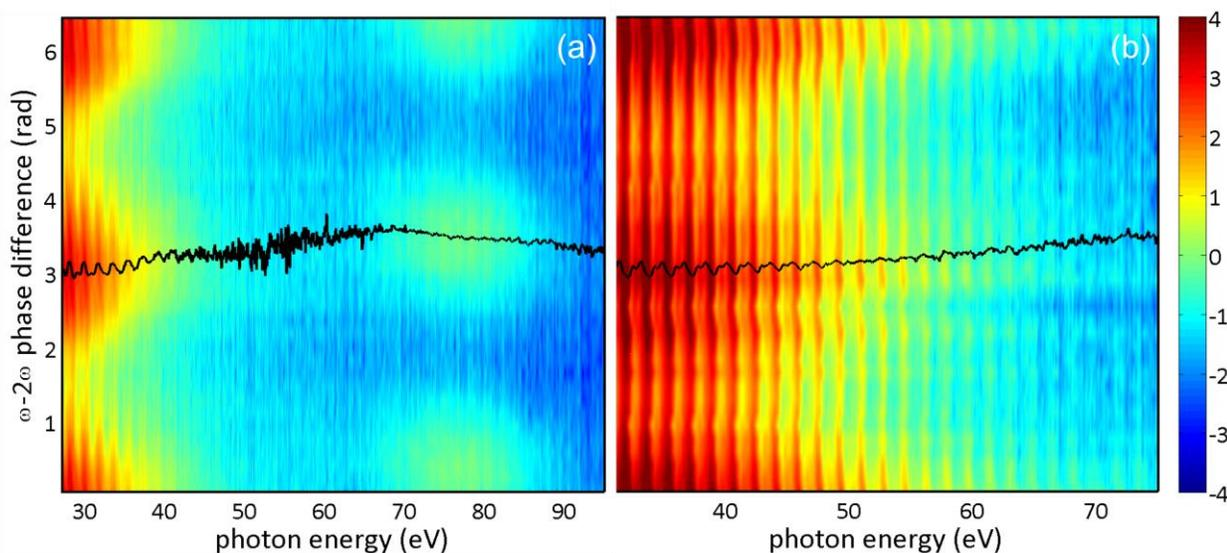
**Figure 1** Scan of harmonic spectra acquired in xenon (a) and krypton (b) as a function of photon energy and two-color phase difference (log scale). The black line corresponds to the phase of the spectral oscillation retrieved by Fourier transforming the sequence of harmonic spectra for each photon energy and by selecting the component at the oscillation frequency.
