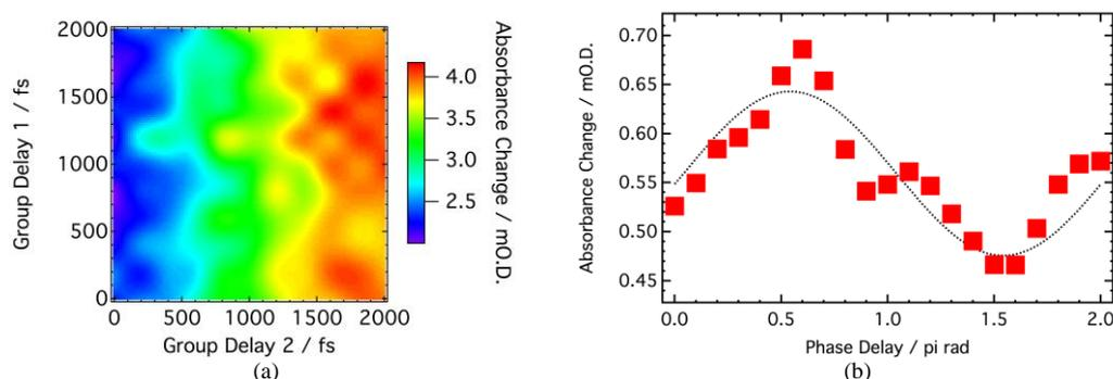
**Fig. 3** (a) Absorbance change for  $|1_S 1_A\rangle$  to  $|2_S 1_A\rangle$  transition plotted against group delays 1 and 2. (b) The phase  $\phi_4$  dependence of the absorbance change for the  $|1_S 1_A\rangle$  to  $|2_S 1_A\rangle$  transition.
