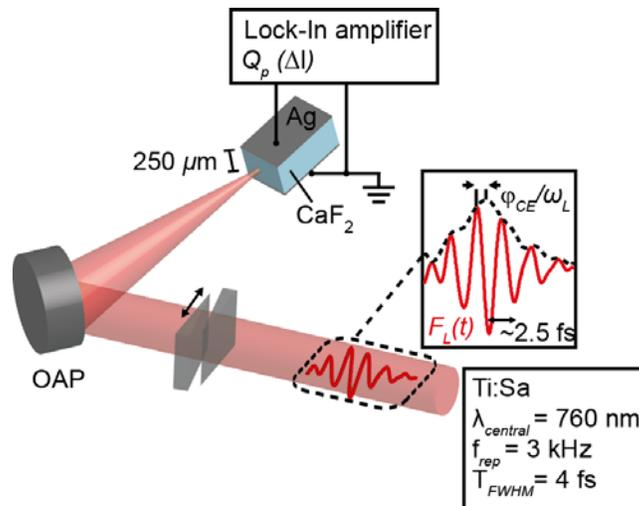
Fig. 1. Experimental Setup, adapted from [4]. The edge of a 250 μm thick dielectric substrate is illuminated by few-cycle Ti:Sapphire pulses at a repetition rate of 3 kHz. The beam is polarized perpendicularly to the gap formed by two silver electrodes and focused down to about 60 μm ( $1/e^2$ ), providing electric field strengths of a few V/Å. The CEP-dependent transferred charge is measured with a lock-in amplifier.
