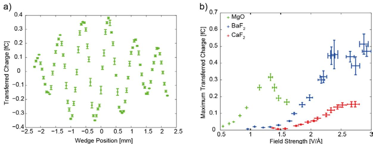
Fig. 2. Laser-Induced Transferred Charge. a) The transferred charge per pulse averaged over 1,500 shots shows a clear dependence on the position of the pair of fused silica wedges used to adjust the carrier envelope phase of the pulse. b) The signal amplitude as well as the critical field strength at which the signal sets in depends on the band gap of the material. The increase of the maximum transferred charge is shown for  $\text{MgO}$ ,  $\text{BaF}_2$ , and  $\text{CaF}_2$ .
