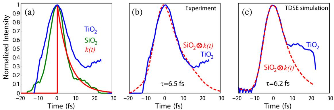
**Fig. 2** (a). Retrieved intensity envelopes from the measured FROG traces. Blue: titania. Green: silica. Red: kernel function employed in deconvolution. (b) Titania envelope in comparison with convolved silica envelope. Time constant was chosen to match the response near zero delay. The lasting component appears to stem from free carriers. (c) Same as in (b), but for numerical results of the TDSE.
