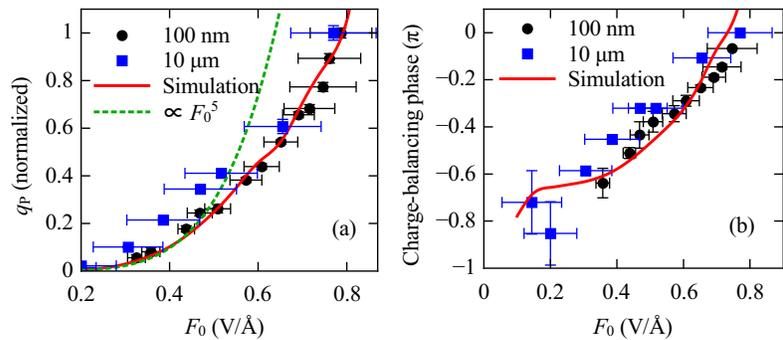
Fig. 2. (a) Dependence of transferred charge on the laser field amplitude. The measurements were done for different distances between the electrodes ( $d = 100$  nm and  $10 \mu\text{m}$ ), and the simulations were performed according to Ref. [2]. (b) Intensity-dependent phase  $\varphi_{CE}^{(0)}$ , which yields a zero transferred charge.
