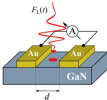
Fig. 1. A schematic picture of the sample: gold electrodes separated by distance  $d$ , fabricated on the GaN substrate.
