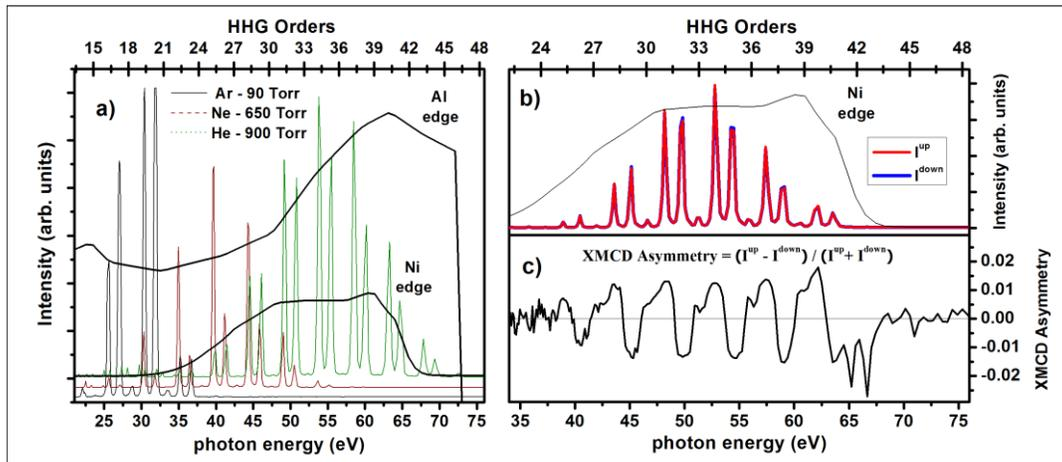
Figure 2 – a) Spectra of bright circularly-polarized HHG in Ar, Ne and He & b), c) XMCD of 50 nm Ni from HHG in He.
