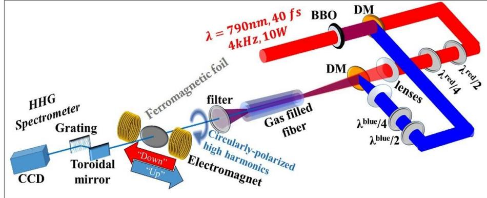
Figure 1 - Setup for generating circularly-polarized harmonics under phase-matching conditions.
