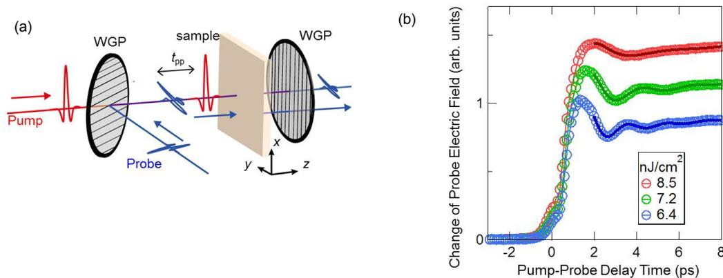
Fig. 2. (a) A schematic picture of the THz pump-THz probe spectroscopy. (b) Experimentally observed temporal evolution of the change of the probe THz electric field at 4 K at the indicated pump intensities. The damped oscillation fits are shown by solid lines.
