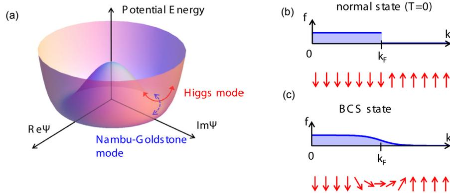
Fig. 1. (a) A schematic picture of the phase mode (blue arrow) and the Higgs amplitude mode (red arrow) in terms of free energy. (b),(c) A schematic picture of normal state and superconducting state represented by the Anderson's pseudo-spins.  $k_F$  is the Fermi wave number.
