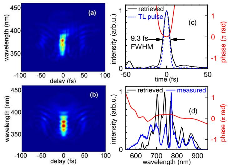
**Fig. 3.** SHG-FROG characterization of the NIR channel: (a) Measured and (b) retrieved FROG traces. (c) FROG retrieved temporal intensity and phase profiles as well as TL intensity profile. (d) Measured spectrum, FROG retrieved spectral intensity and phase.
