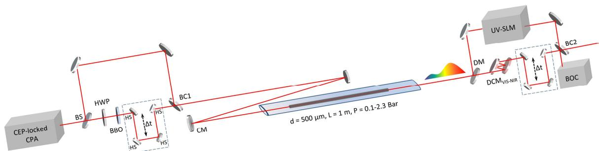
**Fig. 1.** Sub-femtosecond IPM-based optical waveform synthesizer: BS, beam splitter; BBO,  $\beta$ -barium borate crystal; HWP, half-wave plate; HS, harmonic separator; BC, beam combiner; CM, concave mirror; DM, dichroic mirror; DCM, double-chirped mirror; SLM, spatial-light modulator; BOC, balanced optical cross-correlator.
