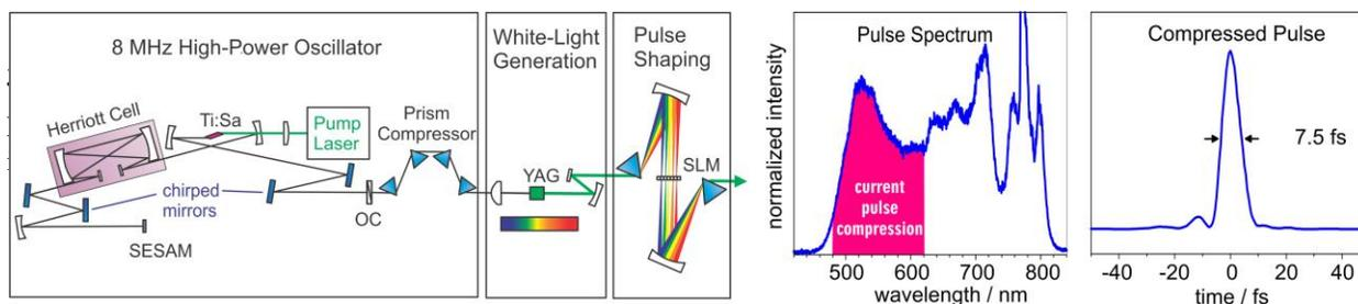
Fig. 1. Setup of the femtosecond white light source, output spectrum, and reconstructed temporal profile of the compressed output pulses. The current spectral range for compression is marked in magenta. Abbreviations: SESAM: Semiconductor saturable absorber mirror. OC: Output coupler. SLM: Spatial Light Modulator.
