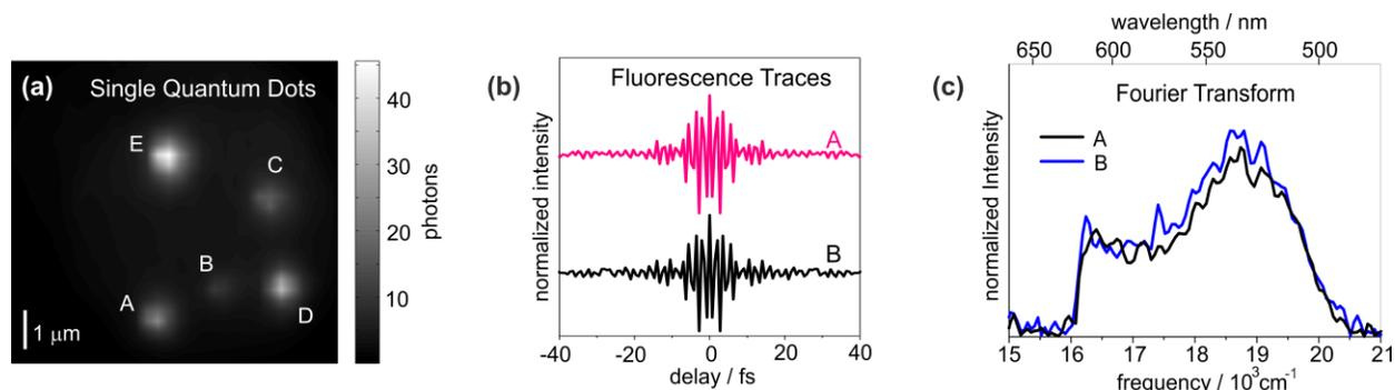
Fig. 2. Femtosecond experiments on single quantum dots. (a) Wide-field fluorescence image of single quantum dots (QDot 655 from Invitrogen) on a glass surface. (b) Delay-dependent fluorescence intensities of two individual dots illuminated with a pair of identical transform-limited white-light pulses. For Fourier transformation the traces were mirror-imaged around time zero. (c) Fourier transform spectra of the traces in (b).
