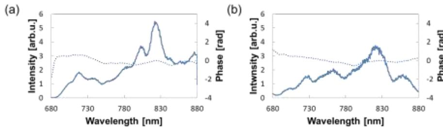
Fig. 3 (a) Measured plasmon spectrum when the excitation polarization was tilted at 45-degree from one of arms of nanocross consisting of nanorods of  $R=2.5$  and  $3.5$ . (b) Calculated plasmon spectrum with the orthogonal response functions shown in Fig. 2 (b).
