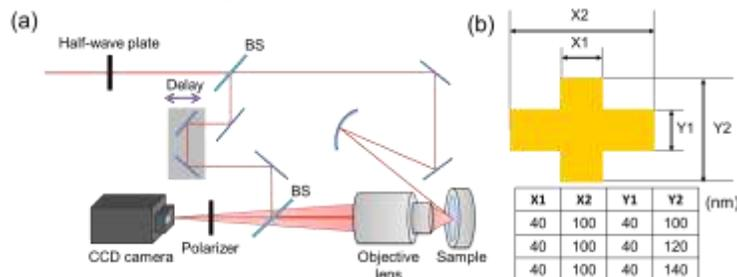
Fig. 1. (a) Experimental setup of dark-field microscopy. (b) Shape of Au cross-shaped nanostructure.
