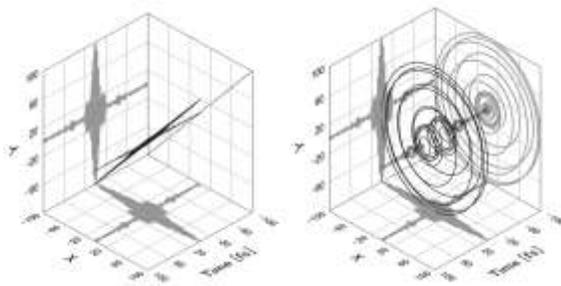
Fig. 4 Vector shaped plasmon pulse based on the orthogonal plasmon response functions.
