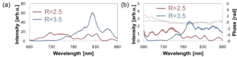
Fig. 2. (a) Plasmon spectra and (b) response functions of nanocross with  $R=2.5$  and  $3.5$ .
