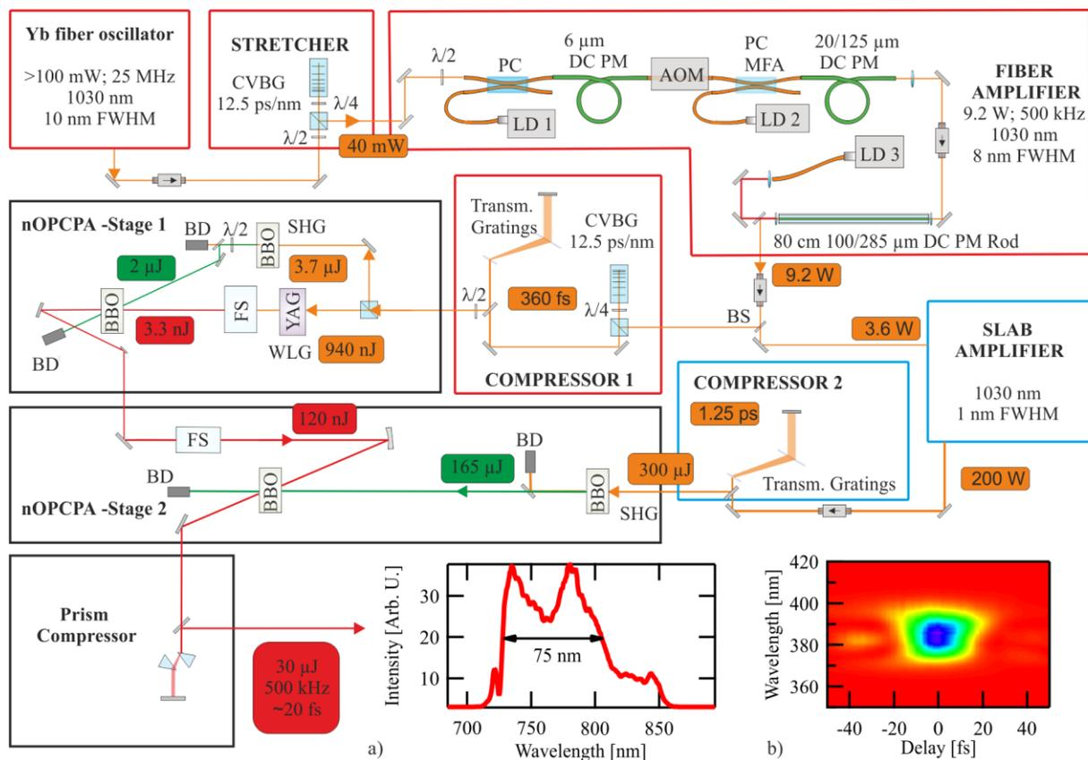
Fig. 1: OPCPA scheme. CVBG Chirped Volume Bragg Grating; LD laser diode; PC pump combiner; MFA mode field adapter; DC PM Double clad polarization maintaining; SHG second harmonic generation; WLW white light generation; FS fused silica. Insets a) Spectrum after the prism compressor b) SHG FROG for the given spectrum
