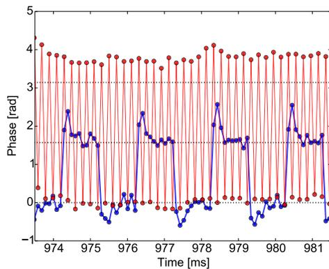
Fig. 1: CEP values acquired at 10 kHz. Red trace and data points: Phase shifter in open-loop configuration. Blue trace: Closed-loop step response. The target CEP is switched by  $\pi/2$  every 10 shots.
