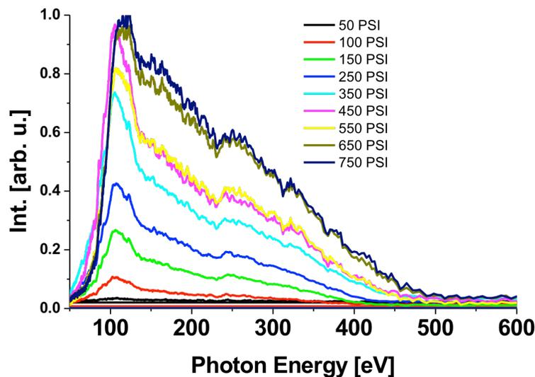
Fig. 1. Harmonic spectra in He for different backing pressure of our pulsed gas cell.
