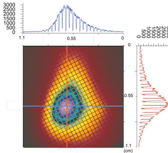
Fig. 2: Beam profile of the X-Ray beam
