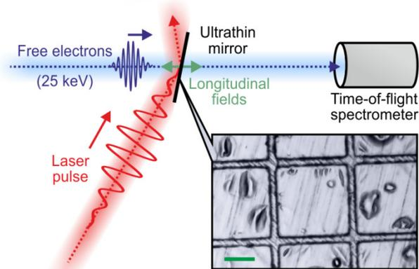
Fig. 1: Concept of the optical-field-driven streak camera for free-electron pulses at 25 keV. The inset shows the 50-nm thin aluminum foil (green scale bar denotes 100  $\mu$ m).
