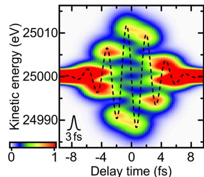
Fig. 3: Semi-classical simulation of free-electron streaking showing sampling of a 5-fs laser field (dashed) with stabilized carrier-envelope phase by a 3-fs free-electron pulse.
