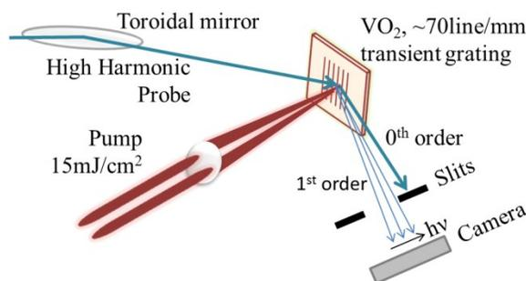
**Figure 1:** Transient grating experiment geometry. A transient grating with ~15 μm period created on the VO<sub>2</sub> surface by two 800nm beams. High harmonics generated in a high pressure gas cell are refocused using a toroidal mirror. First order diffraction from the sample surface is separated from the 0-order beam with slits and detected with a CCD camera.
