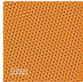
**Figure 1** STM image of the silicene sample
