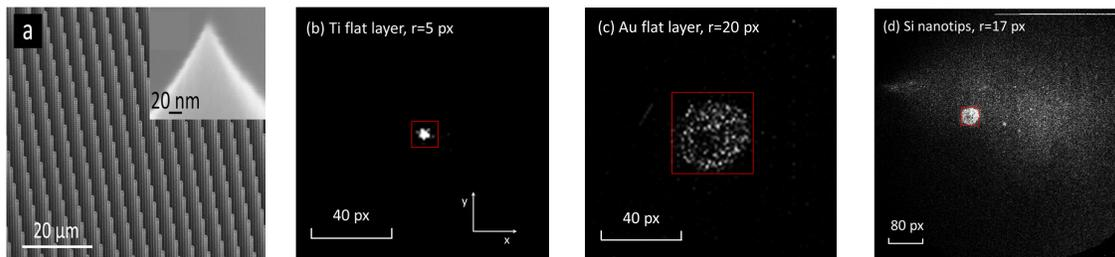
Fig. 2. (a) SEM of the high-aspect-ratio Si-nanotip array; VMI data of (b) flat Ti sample; (c) flat Au sample; (d) Si-nanotip array. The black and white scale represents the relative intensity of electrons detected. The red box indicates the center part of the VMI data.
