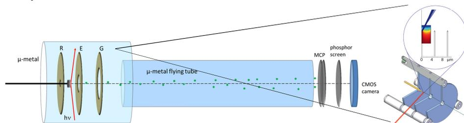
Fig. 1. Configuration of the solid-state VMI. The red solid lines represent the laser beam. R: repeller, E: extractor, G: ground electrode. The green dots represent the emitted electrons.
