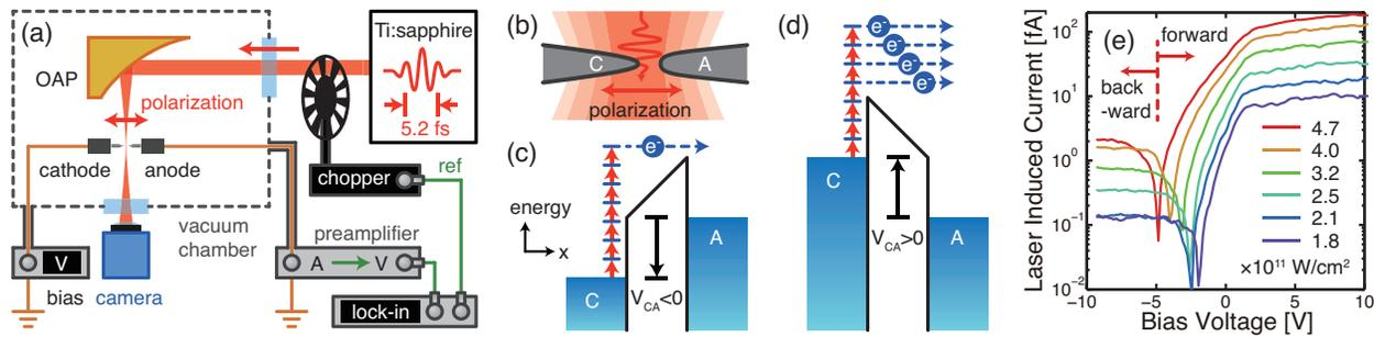
Fig. 1. (a) Schematic of the experimental setup and (b) magnified view around the tip apices (C: cathode, A: anode). Energy diagrams of the laser-injected diode in (c) reverse-bias and (d) forward-bias operations. (e) Current-voltage characteristic curves of the diode triggered by laser pulses with various intensities. Note the current switches sign at the kink in the log-plot.
