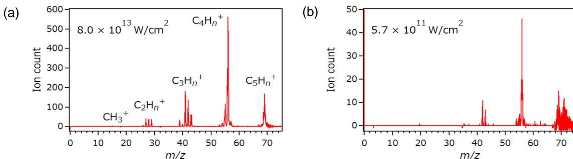
Fig. 3. The mass spectra of the fragment ions generated from the photodecomposition of  $C_6H_{12}^+$  recorded when the laser field intensities were (a)  $8.0 \times 10^{13} \text{ W/cm}^2$  and (b)  $5.7 \times 10^{11} \text{ W/cm}^2$ .
