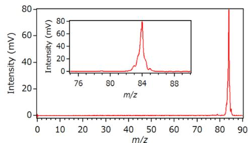
Fig. 2. The mass spectrum of stored ions in the ion trap after the mass selective ion accumulation for C<sub>6</sub>H<sub>12</sub><sup>+</sup> ( $m/z = 84$ ). Inset: the expanded view around  $m/z = 84$ .
