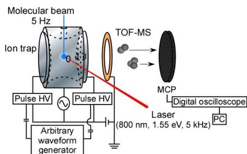
Fig. 1. The schematic of the ion trap TOF-MS.
