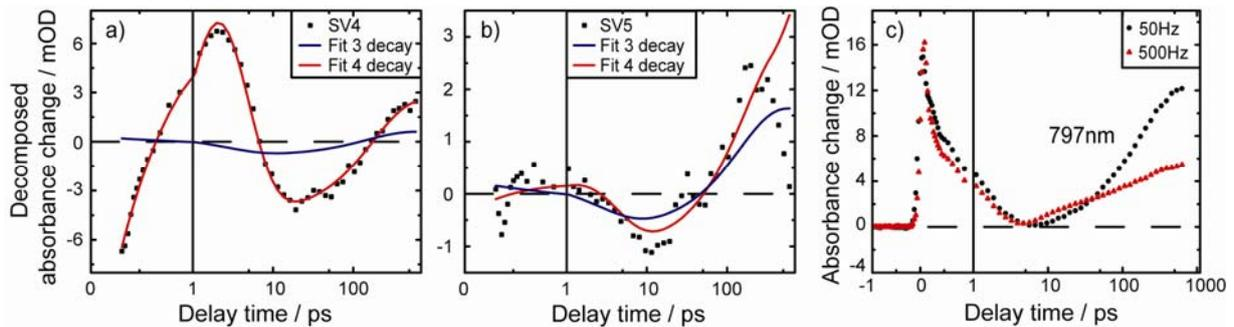
Figure 1: Decomposed transient signal for measurements with 50Hz rep. rate corresponding to the 4<sup>th</sup> SV (a) and 5<sup>th</sup> SV (b). Transient absorption signal at 797nm measured with different repetition rates (c). Displayed data has parallel polarization. The time scale is linear until 1ps and logarithmic afterwards.
