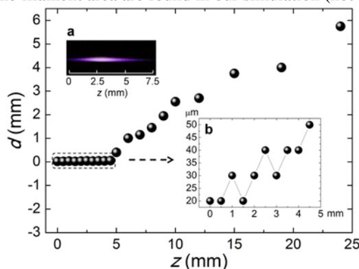
Fig. 3. THz beam diameter  $d$  as a function of  $z$ .
