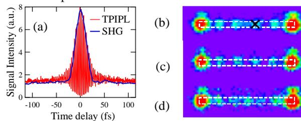
Fig. 2 (a) Time-resolved TPI-PL signal measured at the position  $\times$  in (b) and envelope of SH autocorrelation from BBO crystal. (b,c,d) Transient TPI-PL image of a gold nanorod at the time delay of (b) 0 fs, (c) 19.8 fs and (d) 21.2 fs. Dashed lines represent the outlines of the rod.
