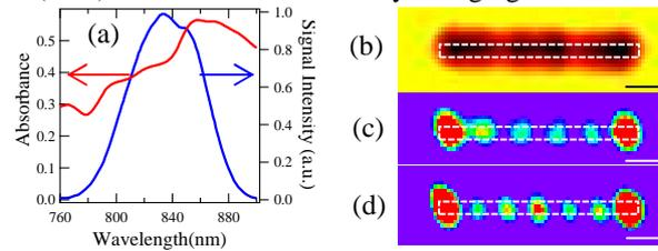
Fig. 1 (a) Near-field absorption spectrum and spectral profile of the irradiated pulses. (b) Near-field transmission image of the gold nanorod probed at 865 nm. (c, d) Near-field two-photon excitation images of the same nanorod excited at (c) 870 nm and (d) 800 nm. Dashed lines represent the outlines of the rod. Scale bar: 200nm.
