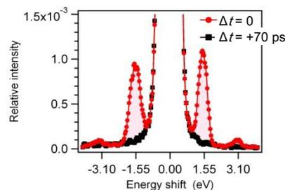
Fig.2. Kinetic energy spectra of scattered electrons by  $\text{CCl}_4$  at  $\Delta t = 0$  (red circles) and  $\Delta t = +70$  ps (black squares).
