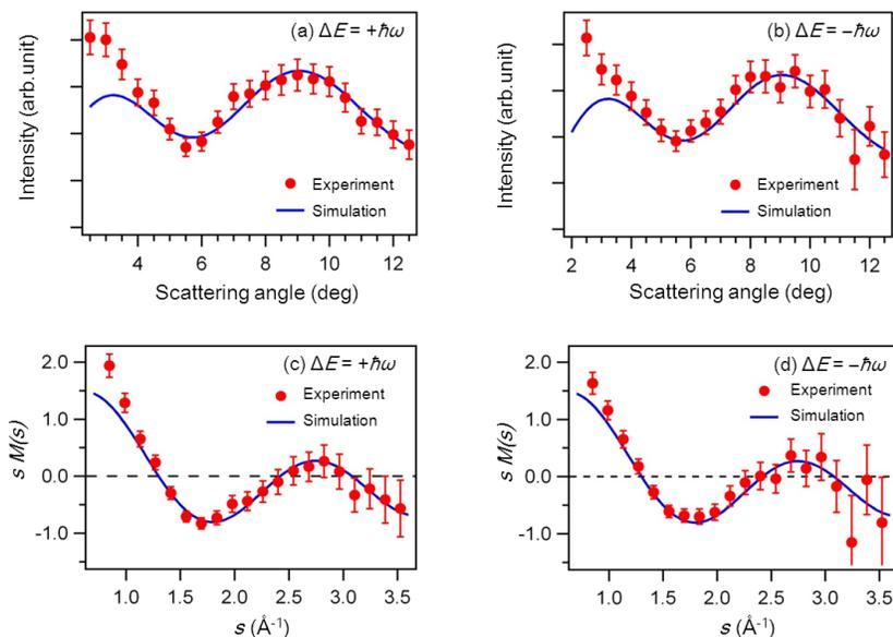
Fig. 3. Upper panels: laser-assisted electron diffraction pattern of  $\text{CCl}_4$  at  $\Delta E = +\hbar\omega$  (a) and at  $\Delta E = -\hbar\omega$  (b). Lower panels: modified molecular scattering intensities calculated from the LAED patterns at  $\Delta E = +\hbar\omega$  (c) and at  $\Delta E = -\hbar\omega$  (d). Filled circles: experimental data. Solid curves: results of the simulation.
