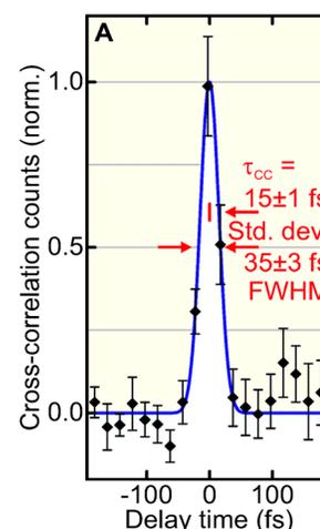
Fig. 1: Shortest electron pulses at 25 keV for atomic-scale diffraction.
