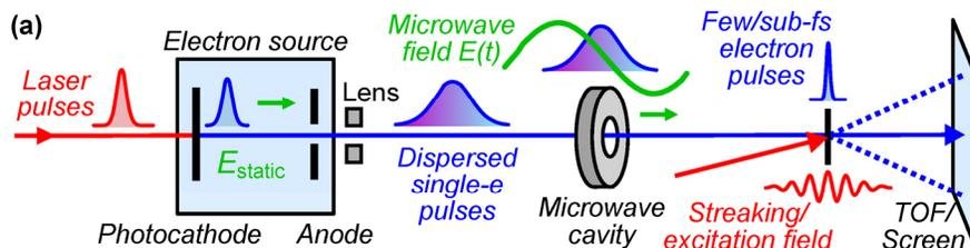
Fig. 2: Single-electron diffraction at ultimate temporal resolution. (a) Experimental concept. (b) Diffraction with compressed single-electron pulses from a molecular switch compound.
