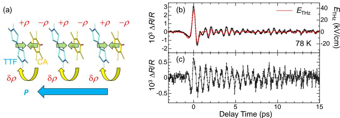
Fig. 1. (a) Schematic of ferroelectric polarization in TTF-CA. (b) THz electric field (red line) and reflectivity change (black line). (c) Oscillatory component of reflectivity change.
