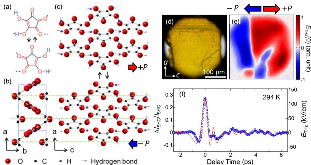
Fig. 2. (a) Molecular structure of  $\text{H}_2\text{C}_5\text{O}_5$ . (b) and (c) show crystal structure of  $\text{H}_2\text{C}_5\text{O}_5$ . (d) Visible image of a  $\text{H}_2\text{C}_5\text{O}_5$  sample. (e) Polarization image of (d) obtained by THz radiation. (f) THz electric field (red line) and SHG intensity change (blue circles).
