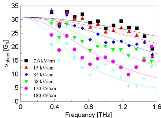
Fig. 2. Symbols: Measured (real-valued) conductivity spectra of graphene at different THz peak field strengths. Lines: fits of the measured THz conductivity to our thermodynamic model, taking into account reduced scattering for hot electrons. The conductivity is shown in quantum units of  $G_0 = e_0^2 / (4h)$ .
