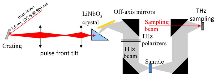
Fig. 1.: The schematic of the nonlinear THz spectroscopy setup used for contact-free ultrafast frequency-resolved current-voltage characterization of graphene.
