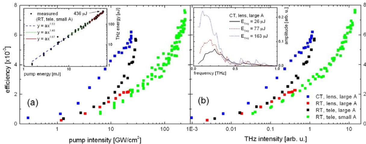
Fig. 1. (a) Measured THz generation efficiency vs. pump intensity (legend: see right panel). Inset: Measured THz energy vs. pump energy. (b) Measured THz generation efficiency vs. THz intensity. Inset: THz spectra obtained from the measured waveforms.
