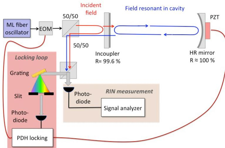
Fig. 1. Schematic of the experimental setup of locking an external optical resonator to the fiber oscillator.
