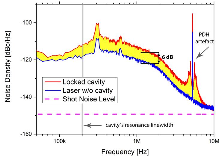
Fig. 2. Noise density of the laser without the effect of the cavity filter (blue curve) and for the case of the locked cavity (red curve). The additional noise is given by the difference (yellow area). The grey vertical line highlights the external resonator's linewidth.
