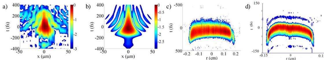
**Fig. 2.** Comparison between the a) experimental and b) simulated spatiotemporal maps at the focus of a diffractive lens. Spatiotemporal maps of c) 100 fs and d) 30 fs FTBs at a distance of 200 mm from the DOE (same color scale as in panel a) applies to c) and d)).
