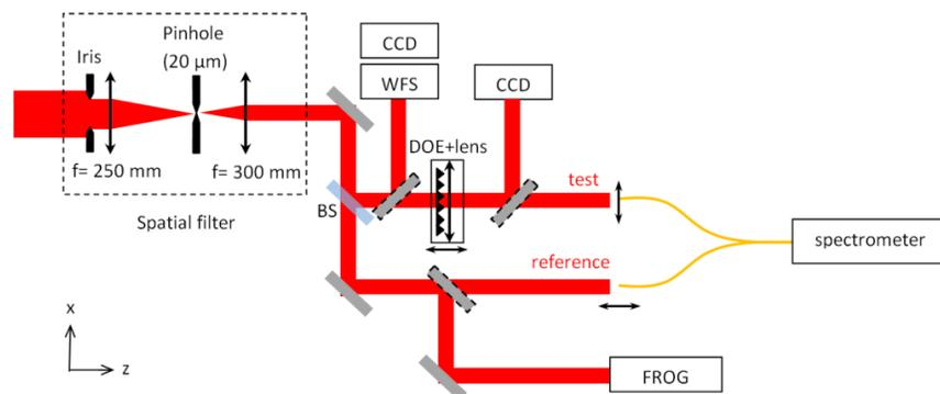
**Fig. 1.** Experimental setup for the spatiotemporal characterization of diffractive shaped beams (see details in the text).
