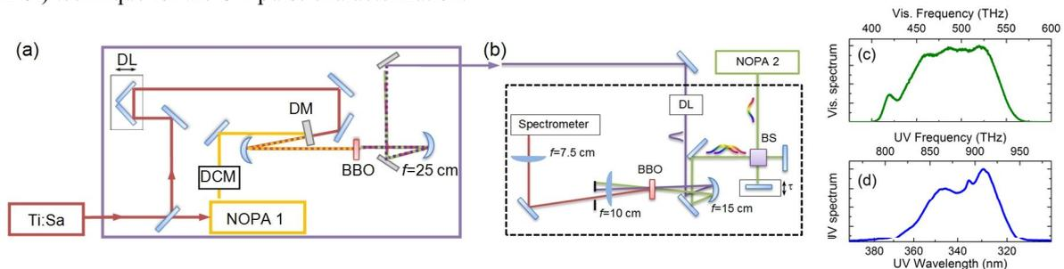
**Fig. 1.** (a) Experimental setup for the generation of UV pulses; DL: Delay Line; DM: Dichroic Mirror; (b) 2DSI setup based on DF generation with an external pulse; BS: cube Beam Splitter. (c) Spectrum of the Visible NOPA1; (d) Spectrum of the UV pulse
