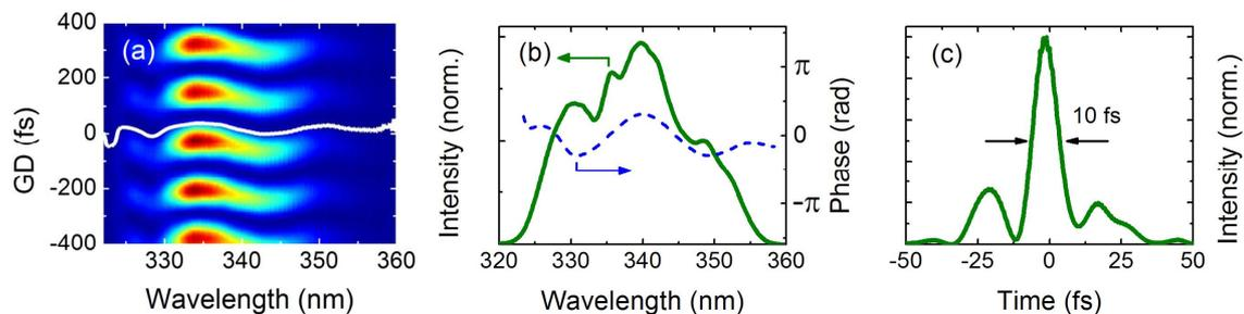
**Fig. 2** (a) 2DSI experimental map and retrieved GD (white line). (b) Spectral intensity (solid) and phase (dashed); (c) retrieved pulse profile.
