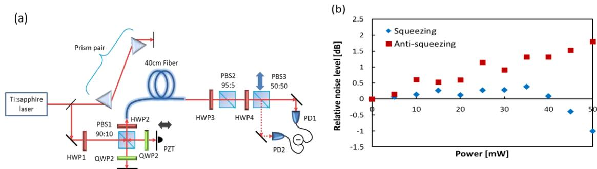
Fig. 2 (a) Experimental setup for generation of photon-number squeezed state by Ti:sapphire laser. HWP: half wave plate, PBS: polarization beam splitter, QWP: quarter wave plate, BS: 50:50 beam splitter, PZT: piezoelectric transducer. (b) Plots of intensity noise relative to the SNL as a function of laser power coupled in to the fiber.
