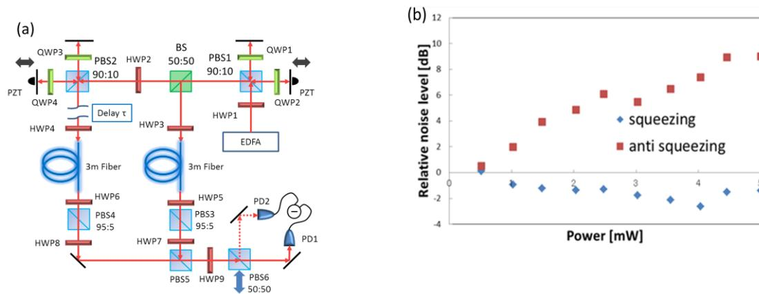
Fig. 1 (a) Experimental setup of CBD-photon number squeezing with EDFA laser using the nonlinear polarization interferometer. HWP: half wave plate, PBS: polarization beam splitter, QWP: quarter wave plate, BS: 50:50 beam splitter, PZT: piezoelectric transducer. (b) Plots of intensity noise relative to the SNL as a function of laser power coupled in to the fiber.
