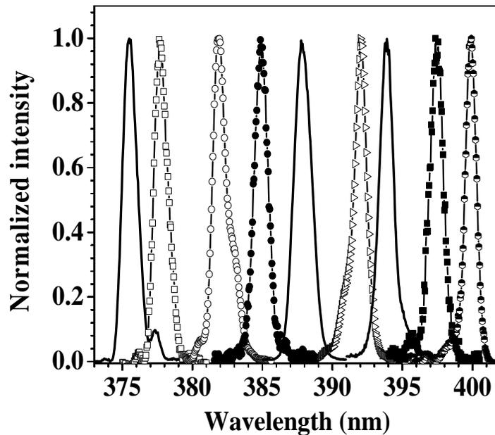
**Fig. 2.** Experimentally recorded sum frequency signals for various phase matching angles from  $31^\circ$  to  $28^\circ$ . For brevity, several measured spectra have been omitted between every two spectra presented here.
