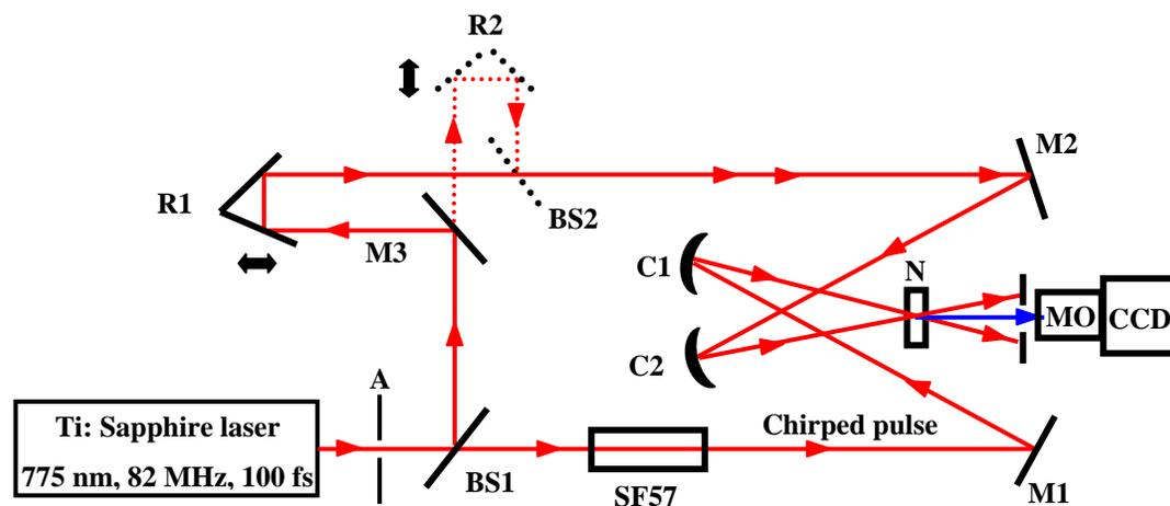
**Fig. 1.** Experimental set up for chirped sum -frequency generation scheme: BS1, BS2 - Beam splitters, A-Aperture, SF57-Glass block, M1, M2, M3-Plane mirrors, R1, R2-Retro reflectors, C1, C2 -Concave mirrors, N-Nonlinear crystal (BBO), MO-Monochromator, CCD-Charge-coupled device. The dotted part of the optical set up is used in for characterization of the pulse. The double arrows ( $\leftrightarrow$ ) indicate the time delay in fs.
