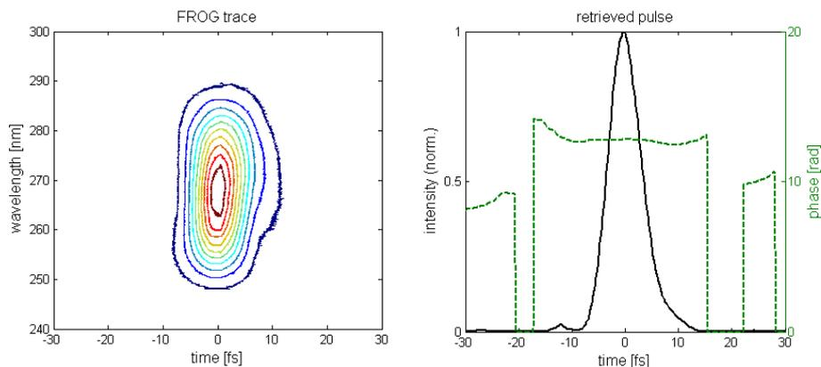
Fig. 2. FROG trace and retrieved temporal profile of pulse (solid) together with its phase (dashed).
