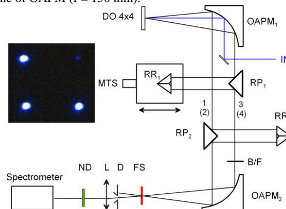
**Fig. 1.** Experimental layout of FROG setup. Inset shows a photograph of incoming beams and FROG-signal (left-upper corner).
