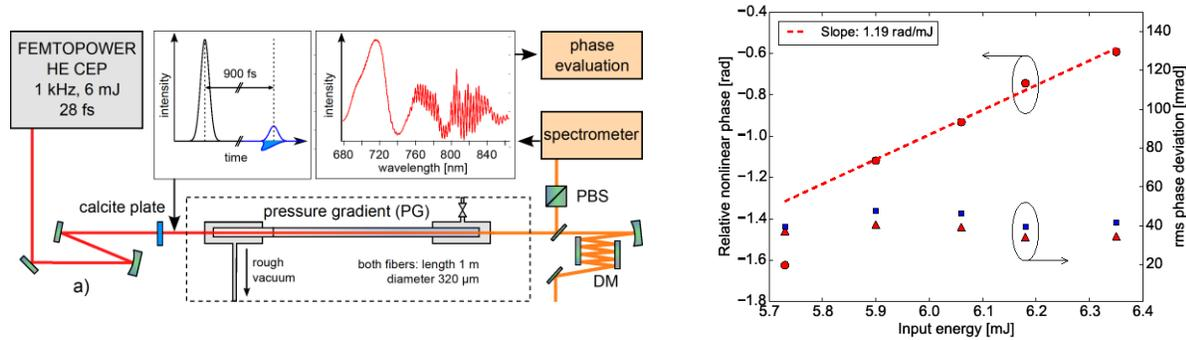
**Figure 1:** a) Experiment setup. See text for details. PBS: polarizing beam splitter cube; DM: dispersive mirror compressor. b) Mean phase change and phase jitter emerging in the HFC. Red circles: mean phase extracted by ISI. Red triangles: rms CEP jitter extracted from the same dataset. Blue squares: rms CEP jitter calculated from shot-to-shot energy fluctuation. The leftmost data point was omitted in the fit, its lower value probably due to decreased gas pressure in the fiber.
