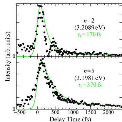
Fig. 2 Observed delay time dependence of the Kerr intensity in a CuCl thin film. The green lines represent the exponential functions convoluted by the excitation laser profile.
