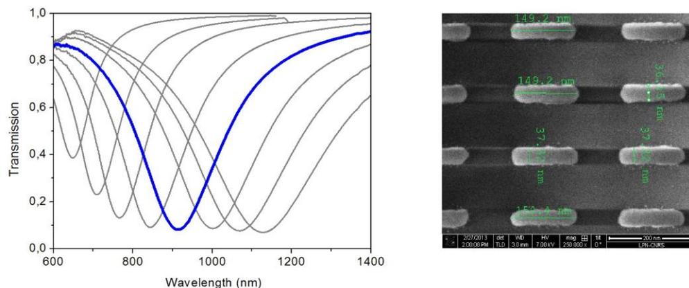
Fig. 1. Left panel: Transmission spectra at the plasmonic resonance for the different gold nanoantennas. Right panel: SEM image of the antenna used in the experiments.
