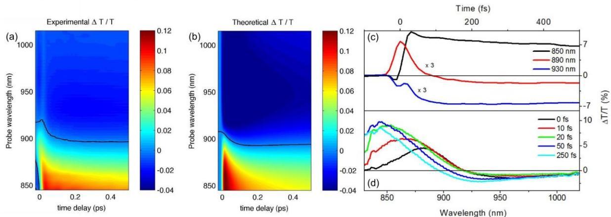
Fig. 2. (a) Pump-probe experimental map for the nanoantenna presented in Fig. 1 as a function of time and probe wavelength and (b) theoretical modeling based on a three temperature model. (c) Dynamics at 850 nm and 890 nm and (d) transient spectra at different pump-probe delays.
