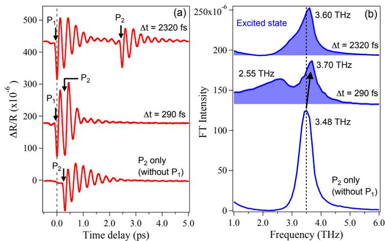
Fig. 1. (a) Transient reflectivity trace observed in the SET phase of SL film at  $\Delta t = 290$  fs and 2,320 fs. The result for the case without prepump ( $P_1$ ) pulse is shown at the bottom for reference. (b) FT spectra obtained from the time-domain data in (a).
