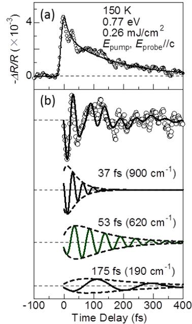
**Fig.3.** (a) Time evolution of  $\Delta R/R$  at 150 K ( $0.26 \text{ mJ/cm}^2$ ) measured by using 12 fs pulse for  $E_{\text{pump}}//c$ ,  $E_{\text{probe}}//c$ . (b) Oscillating components .
