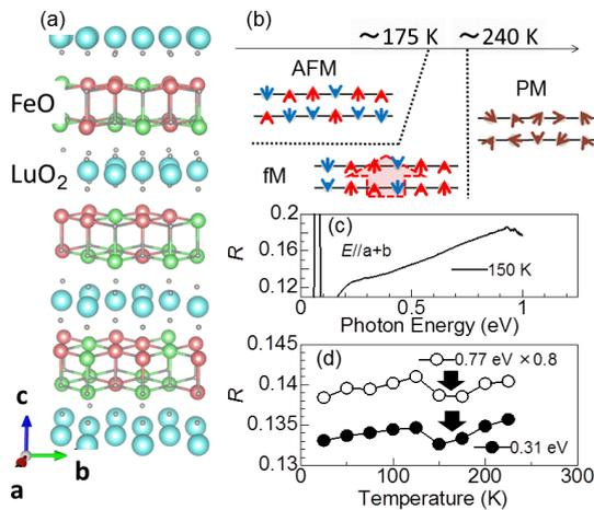
**Fig. 1.** (a) Crystal structure of  $\text{LuFe}_2\text{O}_4$  consisting of FeO double layers and  $\text{LuO}_2$  blocks (b) Schematic illustration of magnetic transition. (c) Steady state reflectivity ( $R$ ) at 150 K. (d) Temperature dependence of  $R$  at 0.77 eV and at 0.31 eV
