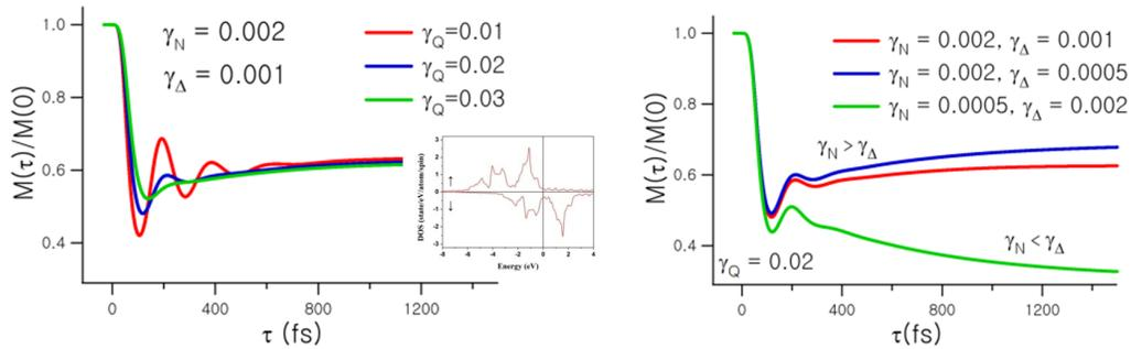
Fig. 1. Time-dependent magnetization of Fe after the ultrashort optical pumping. Inset of the left panel is density of states (DOS) of Fe, adopted in the calculation.
