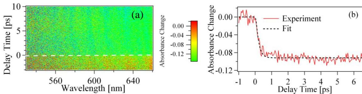
Fig. 2. (a) Time-frequency 2D image of the absorption change obtained in GST. (b) Time evolution of the absorbance change obtained by cutting off the 2D image at  $650 \text{ nm}$ . The solid and dotted lines are experimental data and the best fits to the data, respectively.
