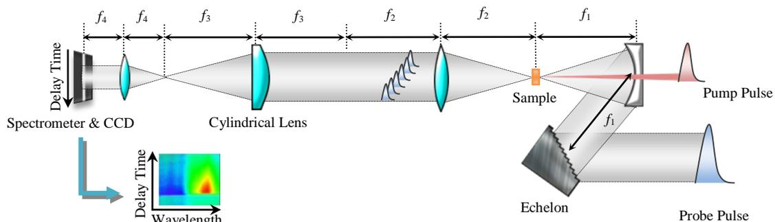
Fig. 1. Schematic configuration of single-shot real-time pump-probe imaging spectroscopy.
