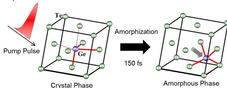
Fig. 3. Diagram of the photo-induced phase-change in GST.
