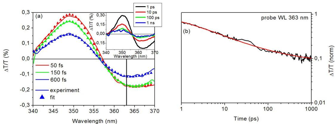
Fig. 2. (a)  $\Delta T/T$  spectra at different pump-probe delays for the  $S_{33}$  exciton, following excitation at  $S_{11}$ , together with a fitting model based on the energy shift contribution from Stark effect. (b) Dynamics at 363 nm for excitation at  $S_{11}$  and fitting with a  $t^{-0.5}$  power law.
