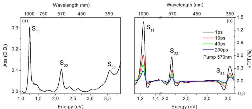
Fig. 1. (a) Ground state absorption spectrum of the (6,5) semiconducting carbon nanotubes used for the experiments. The sharp peaks are due to excitonic transitions, in particular  $S_{11}$  at approximately 1  $\mu\text{m}$ ,  $S_{22}$  at 570 nm and  $S_{33}$  at 350 nm. (b)  $\Delta T/T$  spectra for the (6,5) CNT sample at different pump-probe delays for 570 nm excitation wavelength.
