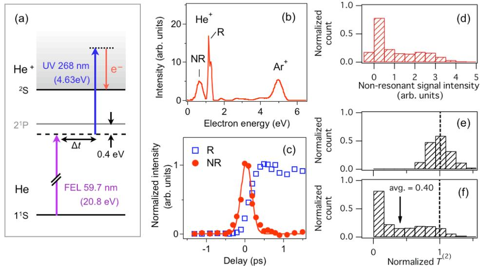
Fig. 1. (a) Schematic diagram of two-color two-photon ionization of He using EUV-FEL and UV laser pulses (b) Photoelectron spectrum at  $\Delta t = 0$  ps. (c) Temporal behavior for resonant (R) and nonresonant (NR) components of the He peak. (d) Histogram of the NR signal at  $\Delta t = 0$  ps. (e) Simulated histogram of  $T^{(2)}(0)$  without the timing jitter. (f) Same as (e), but the timing jitter is included.
