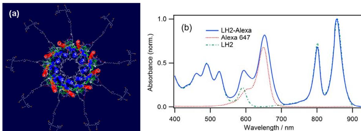
**Figure 1.** (a) Hypothetical image of a LH2 conjugated with nine Alexa Fluor 647. (b) Absorption spectra of LH2-Alexa conjugate (blue solid curve), Alexa Fluor 647 (red dotted curve), and LH2 (green dotted and dashed curve).
