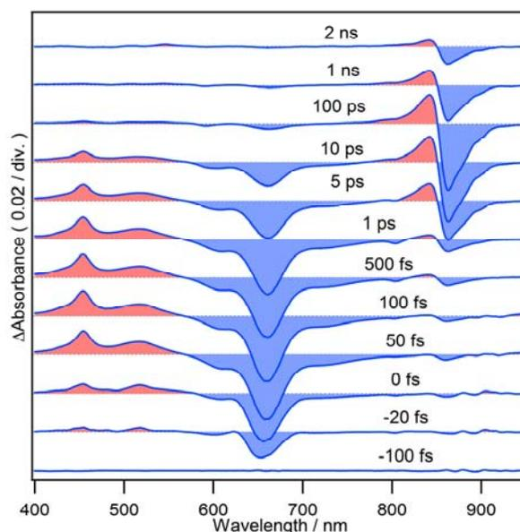
**Figure 2.** Femtosecond transient absorption (TA) spectra of LH2-Alexa conjugate from femtosecond to nanosecond time range excited at 650 nm with pulse duration of 17 fs.
