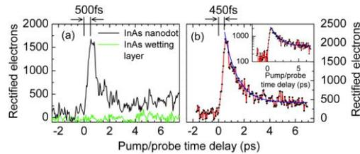
Fig. 2. Optical-pump/THz-STM-probe time scans of ultrafast carrier capture dynamics of single InAs nanodots. (a) Pump-probe time scan with a rise time of the pump-induced signal of about 500 fs. (b) Pump-probe time scan over a different InAs nanodot with a rise time of 450 fs. The blue line is a fit to the data by an exponential decay with a constant offset. The inset shows the same pump-probe response on a semi-log plot. [12]
