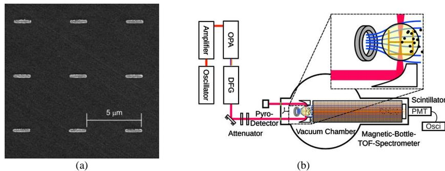
Fig. 1. (a) A scanning electron micrograph of a nanorod array and (b) the experimental setup for photoemission spectroscopy.
