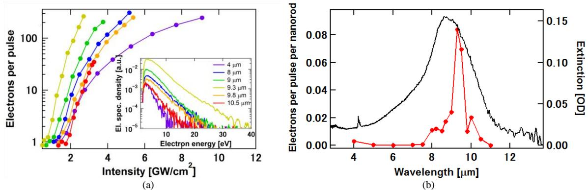
Fig.2. (a) Intensity dependence of electron yields for different excitation wavelengths (inset: kinetic energy spectra measured for constant peak intensity of  $\sim 2.4 \text{ GW/cm}^2$ ). (b) The far-field extinction spectrum for  $2\text{-}\mu\text{m}$ -long nanorods (black) and the photoemission yield (red).
