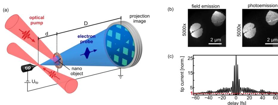
Fig 1: (a) Scheme for femtosecond point projection imaging. (b) Projection images of a 50 nm gold NW lying across  $2 \mu\text{m}$  holes in a free-standing carbon thin film, for field emission and photoemission operation mode, respectively. (c) Interferometric autocorrelation of the nanotip current in the laser-triggered mode.
