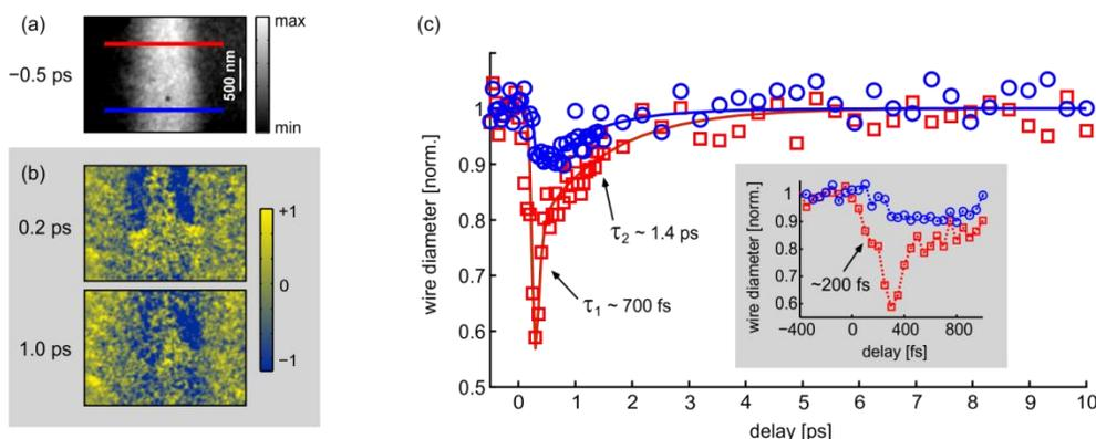
Fig 2: (a) Point-projection image of an InP NW at negative delay times between pump and probe. (b) Transient pump-induced image differences at two selected delay points. (c) Dynamics of the wire diameter in the projection image in two regions of the nanowire indicated with the colored lines in (a). The inset shows the  $\sim 200$  fs initial dynamics of the diameter reduction.
