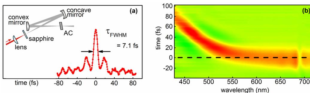
Fig. 2. a) *Schiefspiegler* geometry for imaging the newly generated colors of a 1-mm sapphire continuum and autocorrelation trace demonstrating a 7 fs pulse. b) Transient absorption measurement in 200  $\mu\text{m}$  GG400 to determine the chirp of the continuum generated in a 1-mm sapphire plate.
