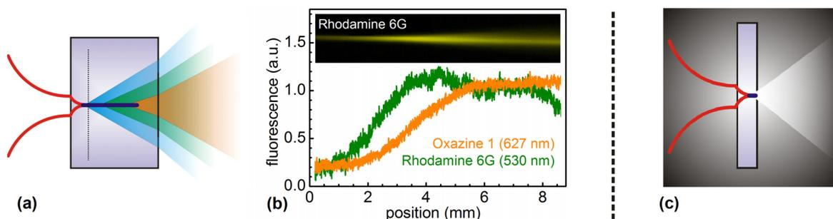
Fig. 1. a) Scheme of bulk continuum generation and wavelength dependent beam propagation. b) Fluorescence of Rhodamine 6G (green) and Oxazine 1 (orange) to monitor the beam propagation during filamentation in ethanol. c) All colors diverge equally in a short crystal.
