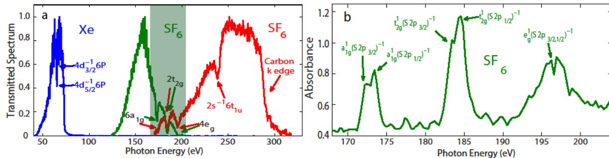
Fig. 2(a) Normalized raw data for 1.3  $\mu\text{m}$ -driven HHG from Ar (blue), Ne (green), and He (red) after transmission through a 2 mm long sample cell of Xe (HHG from Ar), and  $\text{SF}_6$  (HHG from Ne and He). (b) NEXAFS spectrum of  $\text{SF}_6$  Sulfur L-edge 2p orbital.
