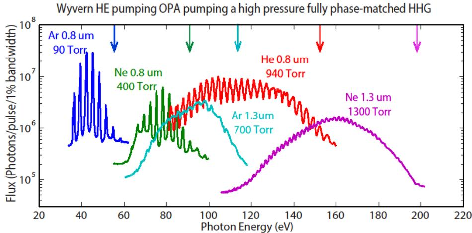
Fig. 1. Flux characterization and comparison of the optimized fully phase matched HHG emission from a 1 cm long, 150  $\mu\text{m}$  diameter, waveguide driven by 1.3  $\mu\text{m}$  and 0.8  $\mu\text{m}$  light in various noble gases (Ar, Ne, and He). The vertical arrows indicate the maximum phase matched HHG energy cutoff for each gas and laser wavelength.
