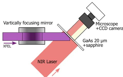
Fig. 1, Top view of the experimental setup for the arrival-timing monitor
