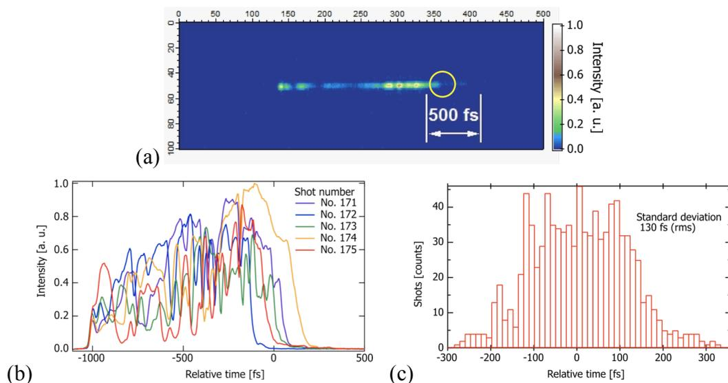
Fig. 2. (a) Transparent image of the NIR laser in the area irradiated with the XFEL beam. (b) Vertical projections of the consecutive images of (a). (c) Histogram of the arrival timing. Standard deviation was 130 fs (rms).
