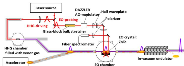
Fig. 1. Experimental setup of seeded FEL with EO-sampling feedback at EUV-FEL accelerator: relative positioning in transverse and timing in longitudinal of electron bunch with respect to arriving timing of a seeding HH pulse are monitored at entrance of the first in-vacuum undulator to keep in a best seeding condition.
