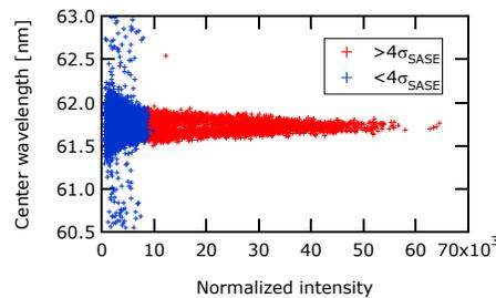
Fig. 2. Correlation data plot between normalized intensity and central wavelength with seeded operation. Here,  $\sigma_{SASE}$  is standard deviation of the SASE-FEL intensity fluctuation. Effective seeded FEL pulses are defined as large as  $4\sigma_{SASE}$  (red) for user experiments.
